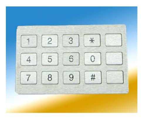
15 keys compact format IP55 dynamic vandal proof Stainless Steel encryption PINPAD with industrial encryption electronics controller supporting DES/TDES shieded & protected by stainless steel housing, industrial PCB with carbon-on-gold key switch technology with long stroke (2.0mm) with extremely good tactile feeling for fast and accurate data input without any noise, top stainless steel plate with threaded bolts under top stainless steel plate for top panel mounting solution.
